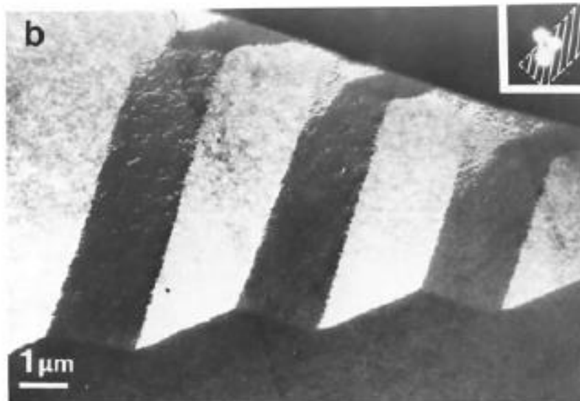
FIG. 27. (a) Defocused image of an Fe-Si alloy specimen showing three magnetic domains. (b) The domain corresponding to spot 3.
